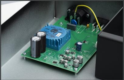
Special Phono Stage PSU Design with Low Core Saturation Toroidal Transformer to Minimize Electromagnetic Radiation
